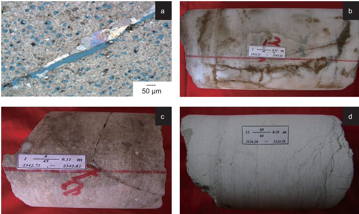
图6 裂缝发育特征 [15] (a)亮晶铸模鲕粒灰岩, 溶蚀缝; (b)垂向扩展缝; (c)构造缝; (d)缝合线 Fig. 6 Fracture characteristics in the study area (a) spray oolitic limestone, dissolution fracture; (b) vertical extension fracture; (c) oblique tectonic fracture; (d) stylolite
