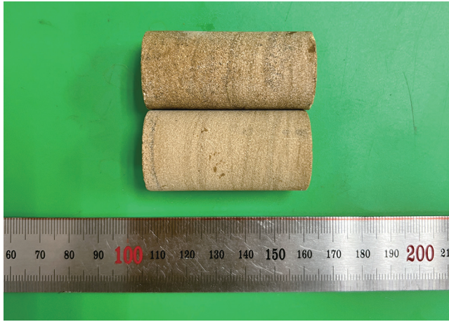
图 15 双轴压缩实验后样品外观图 Fig. 15 Sandstone samples after biaxial compression test
