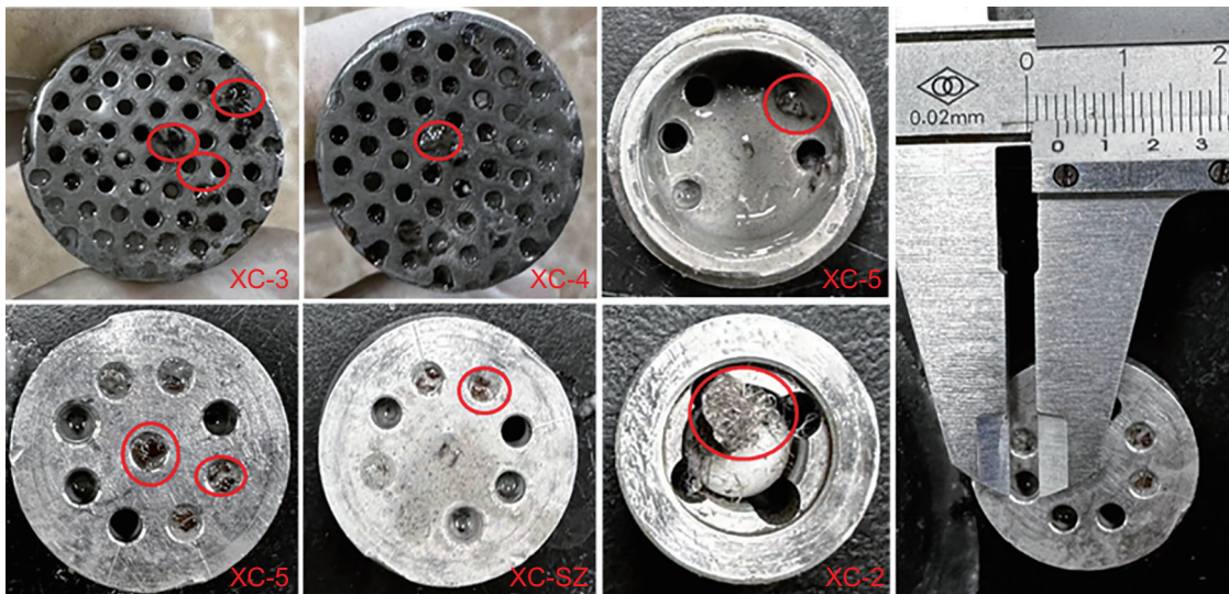
图 9 5 种现场纤维循环后堵塞的网板与仪器配件 Fig. 9 Five kinds of screen plates and instrument accessories blocked by on-site fiber circulation
