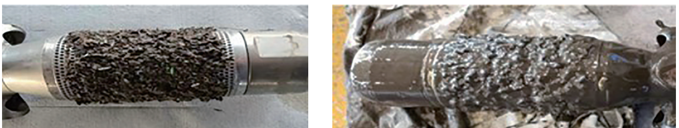
图 10 现场纤维堵塞旋导筛网实物图 Fig. 10 Physical image of on-site fiber blockage rotary screen mesh
